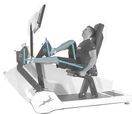
Figure 2: Total range of movement on the DD System. Maximum flexion (right leg) and minimum extension angles (left leg).
